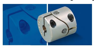
Pin/bushing style couplings that use aluminum alloy as their primary material. This system makes shaft reaction force due to mounting misalignment extremely small. There is also a damping effect from sliding at the friction surface between the pin and dry metal.
