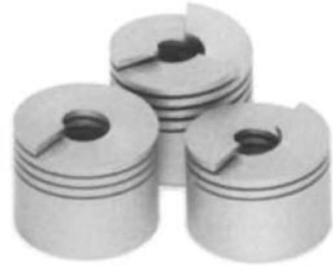
*Multiple, (typically two) helical beams provide high torsional stiffness. Shown: single, double and triple start.*
