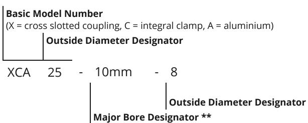
Metric bores are specified as millimetre sizes (-10mm). Inch bores are expressed as number of 32nds (-8=8/32 = 1/4" = .250).
