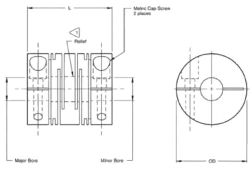
Major and minor diameter shafts may enter flexing area during operation.
