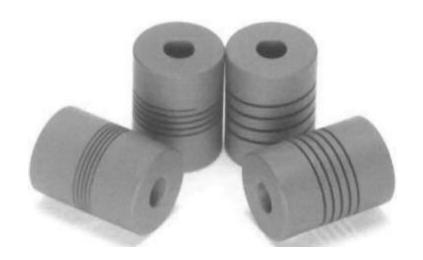
By varying the thickness of the coils, a Flexure can accommodate increasing amounts of torque and radial loads. The designer may specify torsional stiffness and compression spring rates independent of other factors.
