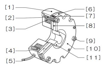
[1]Stator [2]Stud bolt [3]Coil [4]Torque spring [5]Lead wires [6]Armature [7]Auxiliary spring [8]Rotor [9]Hexagon nut [10]Plate [11]Rotor hub
