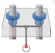
Pressure setting is done with an external pressure source. Several connections can be clamped/ loosened simultaneously.
