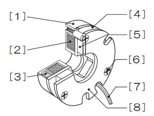
[1]Stator [2]Coil [3]Torque spring [4]Armature [5]Rotor [6]Flat head bolt [7]Lead wires [8]Plate
